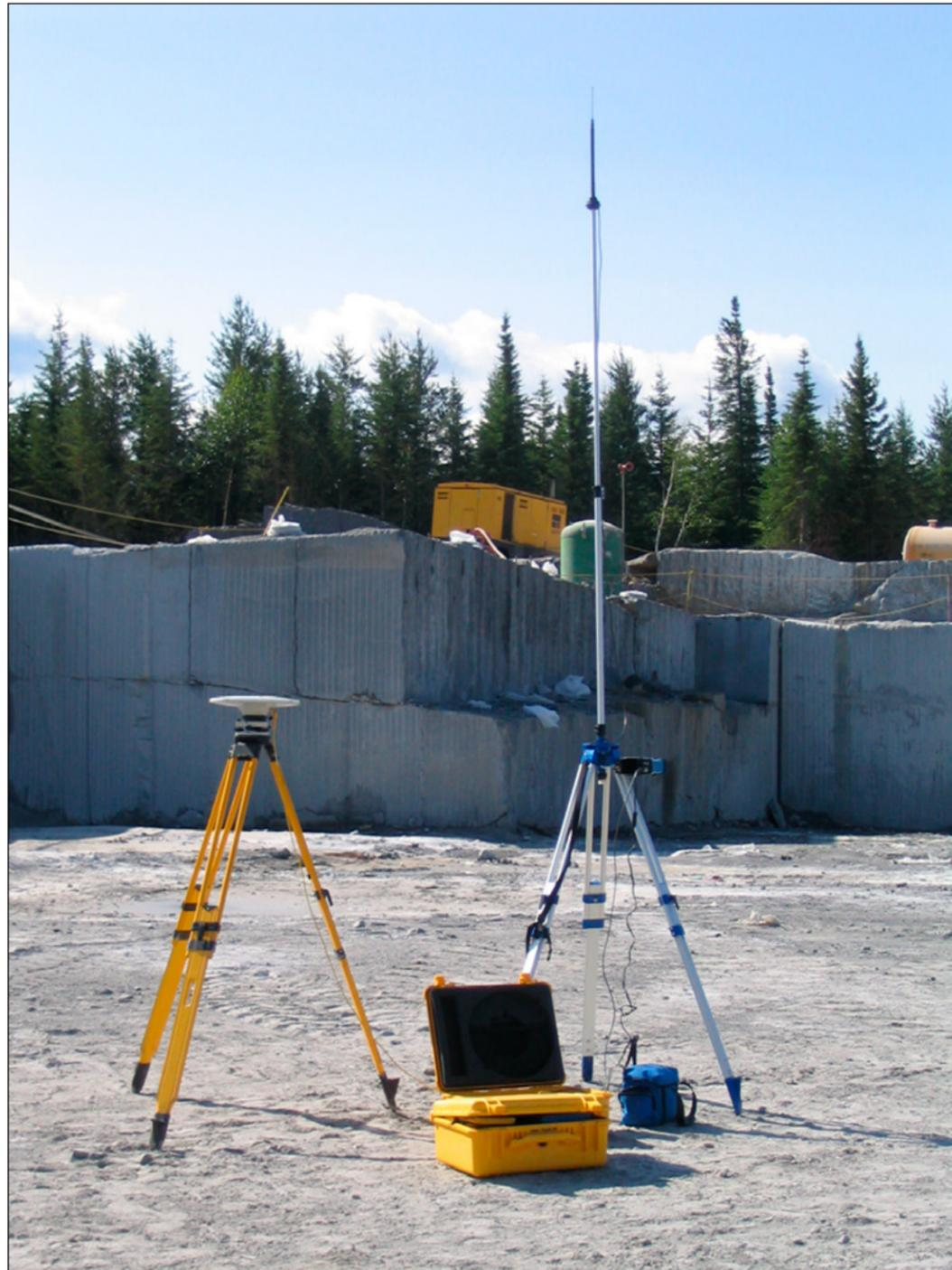
Fig 47. Instruments used for 6-Satellite GPS survey by Bear Island Surveying, Ely, MN, for Latitude, Longitude and Altitude of each slab or block to be installed as part of *SITE INDEX*, in the East and West Gardens and Rosetta Stone. Mesabi Black Quarry, Lake County, MN, May, 2004. Measurements were used to construct the Quarry Block Diagram and determine an accurate quarry site position to be etched into each block for *SITE INDEX*.
