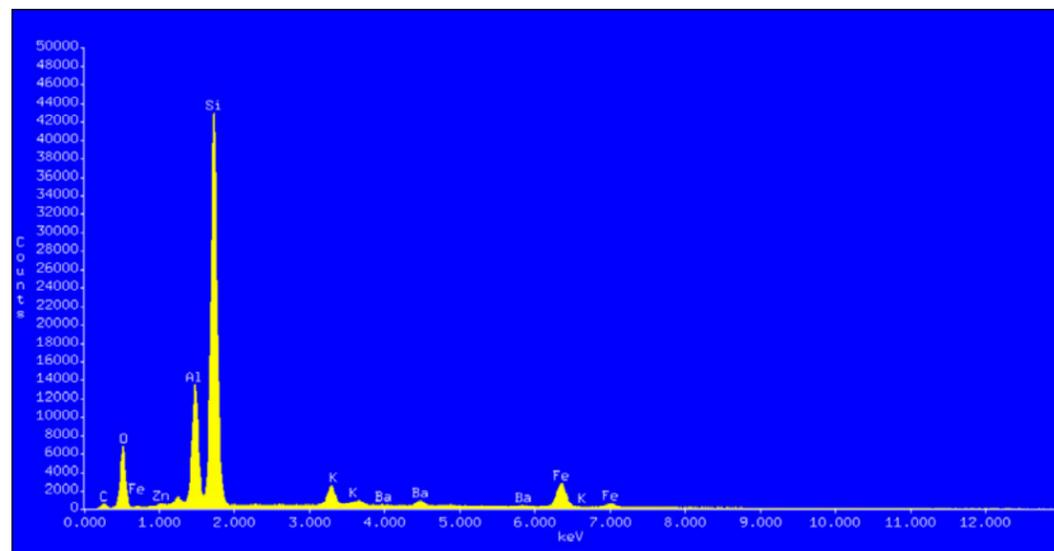
Fig. 96. Brick EDS Data: Accelerating Voltage: 20 KeV - Take Off Angle: 51.3303° - Live Time: 120 seconds - Dead Time: 53.2. Mineral Lab Report 20531, June 3, 2005.
