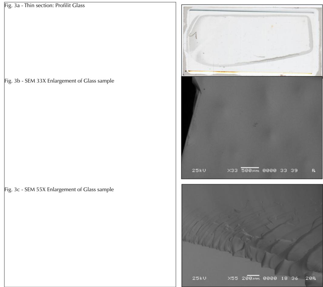
Fig. 124. Thin Section and Scanning Electron Microscopy (SEM) imagery - "Glass" Sample. Mineral Lab Report 20531, June 3, 2005.
