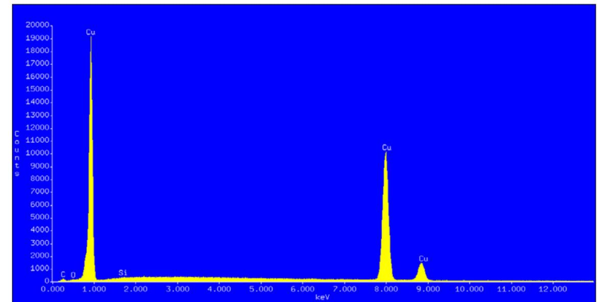
Fig. 133. Copper EDS Data: Accelerating Voltage: 20 KeV Take Off Angle: 52.6559° Live Time: 120 seconds Dead Time: 30.789. Mineral Lab Report 20531, June 3, 2005.
