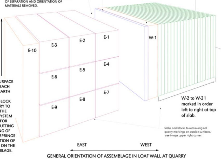
Fig. 51. Ideal Cutting /Quarry Configuration "C" - Mesabi Black Quarry, Ely, MN, one of several studies for the quarrying and cutting of the blocks of anorthositic gabbro for the West, East Gardens and Rosetta Stone.
