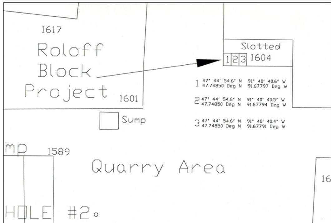
Fig. 49. Roloff Block Project, sketch by Cold Springs Granite based upon Bear Island Survey data, giving GPS location of gabbro blocks to be used for *SITE INDEX*, Rapson Hall gardens. Mesabi Black Quarry, Lake County, MN, 2004.
