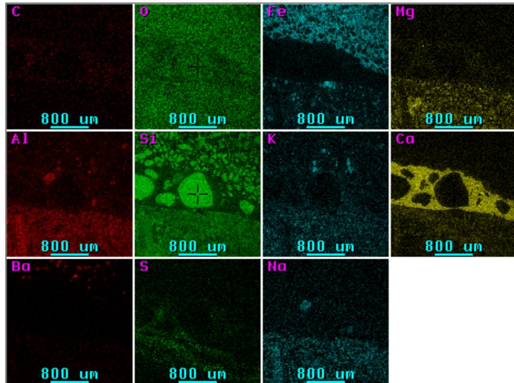
Fig. 105. Concrete Elemental Map Data, Fig. 2b:Accelerating Voltage: 20 KeV - Magnification: 37 - Resolution: 512 x 512 - Pixel Size: 5.20926 microns. Mineral Lab Report 20531, June 3, 2005.
