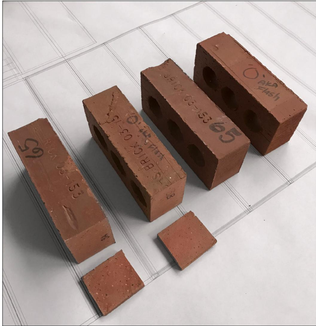
Fig. 93. Anthropocene "Brick" Samples of indurated Upper Cretaceous shale and mudstone, Split Rock Creek Formation, Ochs Brick and Tile Co., 3A and 3B used for testing. Lab no. 20531. Mineral Lab Report, June 3, 2005.
