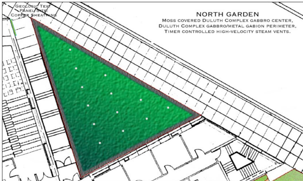
Fig. 65. North Garden, Rapson Hall conceptual study/plan view, moss, crushed gabbro center, gabbro gabion perimeter, steam vents, timer system. Computer graphic by John Roloff on architectural site plan by Steven Holl Architects, 2004.
