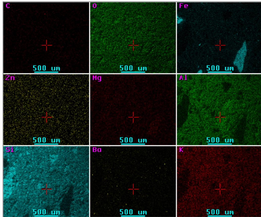
Fig. 95. Brick Elemental Map Data, Fig. 1b: Accelerating Voltage: 20 KeV - Magnification: 55 - Resolution: 512 x 512 - Pixel Size: 3.50441 microns. Mineral Lab Report 20531, June 3, 2005.
