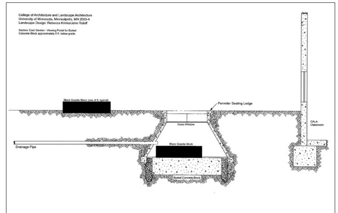
Fig. 74-75. East Garden, Rapson Hall, studies for proposed, *Site Index*, studies for uses of the buried concrete crane pad used in the construction of the Holl Annex. John Roloff computer drawings, 2002-04.
