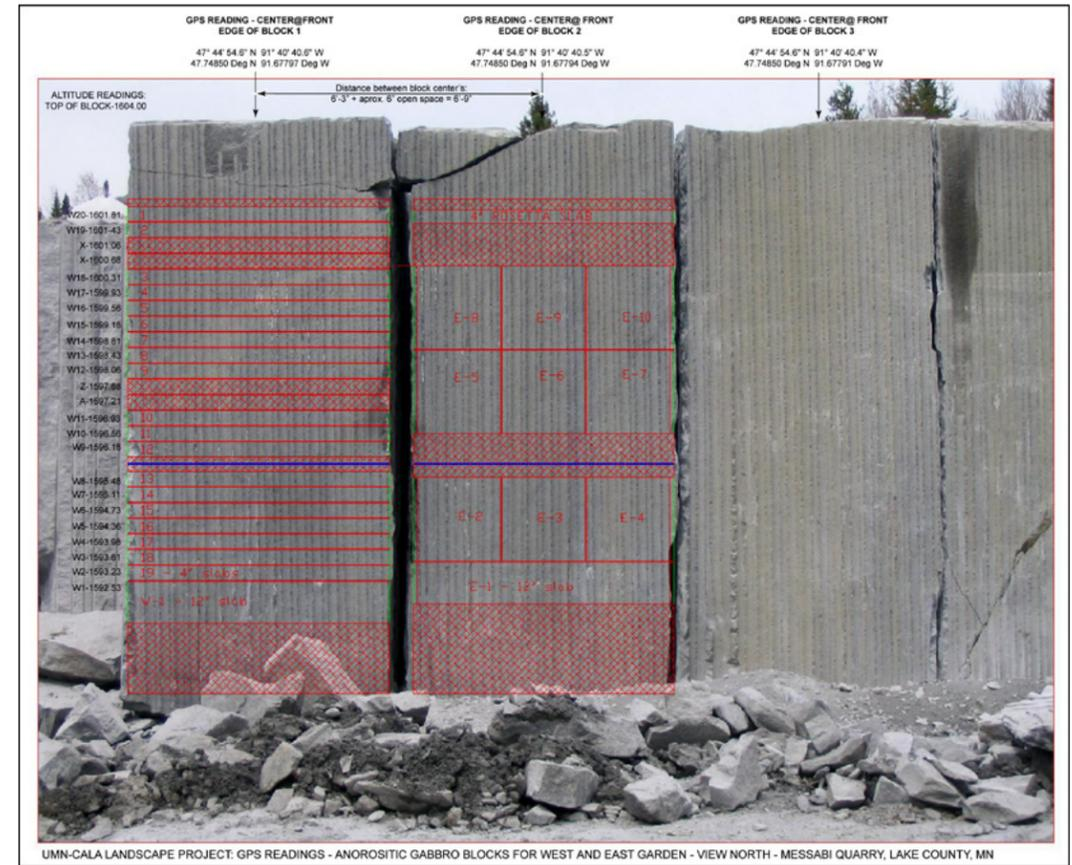
Fig. 50. Cutting diagram based on the GPS altitude, longitude and latitude readings for slabs of anorthositic gabbro to be used for the West Garden (Block 1/W1-20), and East Garden and Rosetta Stone (Block 2/Rosetta and E1-10).
