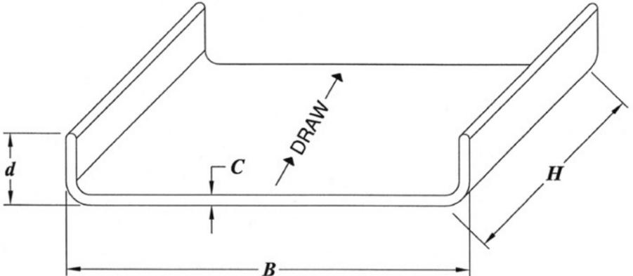
Figure 1. Relationship between U-Channel dimensions and direction of draw.
