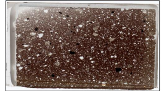
Fig. 1b - SEM 55X Enlargement of Brick sample
