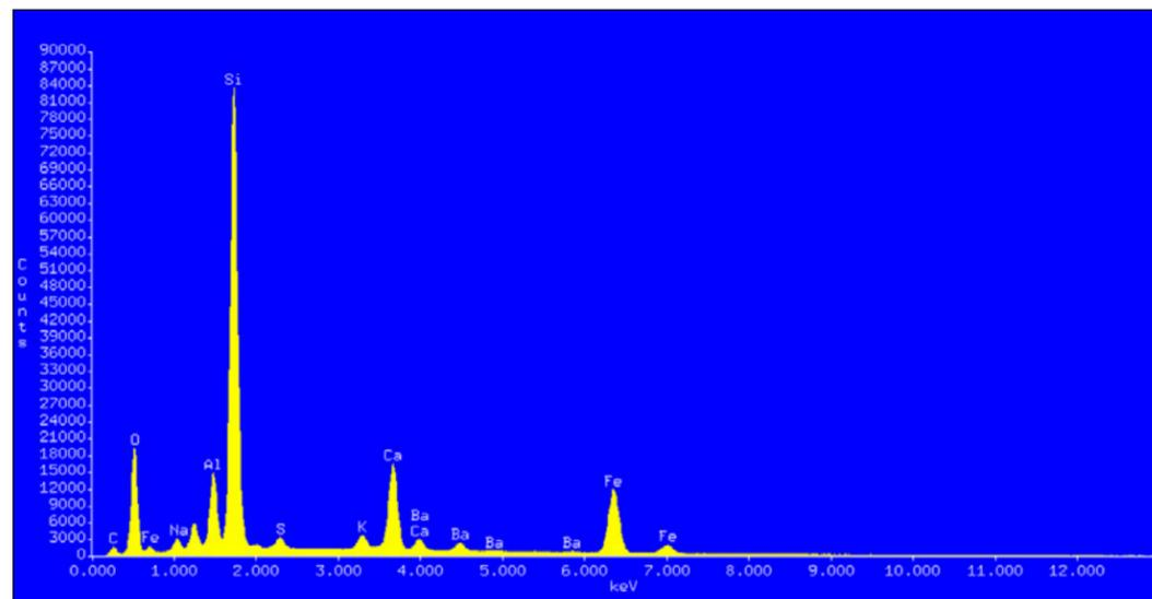
Fig. 106. Concrete EDS Data:Accelerating Voltage: 20 KeV - Take Off Angle: 53.29° - Live Time: 120 seconds - Dead Time: 165.614. Mineral Lab Report 20531, June 3, 2005.
