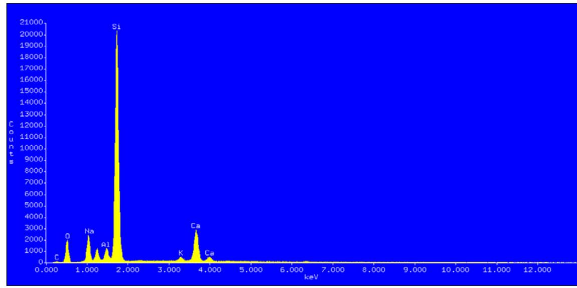
Fig. 125. Glass EDS Data: Accelerating Voltage: 25 KeV - Take Off Angle: 54.504° - Live Time: 120 seconds - Dead Time: 19.157. Mineral Lab Report 20531, June 3, 2005.
