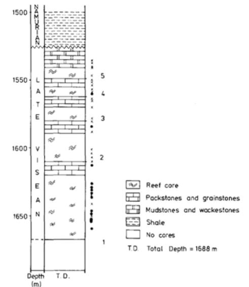
Fig. 3. Log of the Visean limestones in the Poederlee borehole. Superimposed reef mounds are numbered 1 to 5. Black dots next to the log indicate the samples analysed petrographically and geochemically. The crosses indicate samples which have been studied only petrographically.
